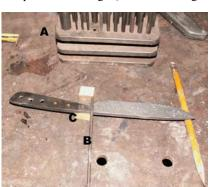
Fg.1: Marking the bolster rivet hole
