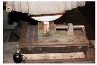
Fg.3: Grinding bolster surfaces
