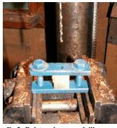
Fg.2: Bolster clamp on drill press
